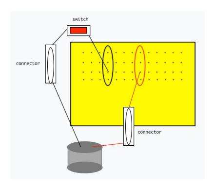
connect red & black wire on the battery and plug into the fourth hole of the breadboard.
