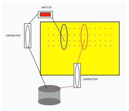
Left side of connector, connect the black wire with the switch and plug into a Third hole(left) of breadboard.
